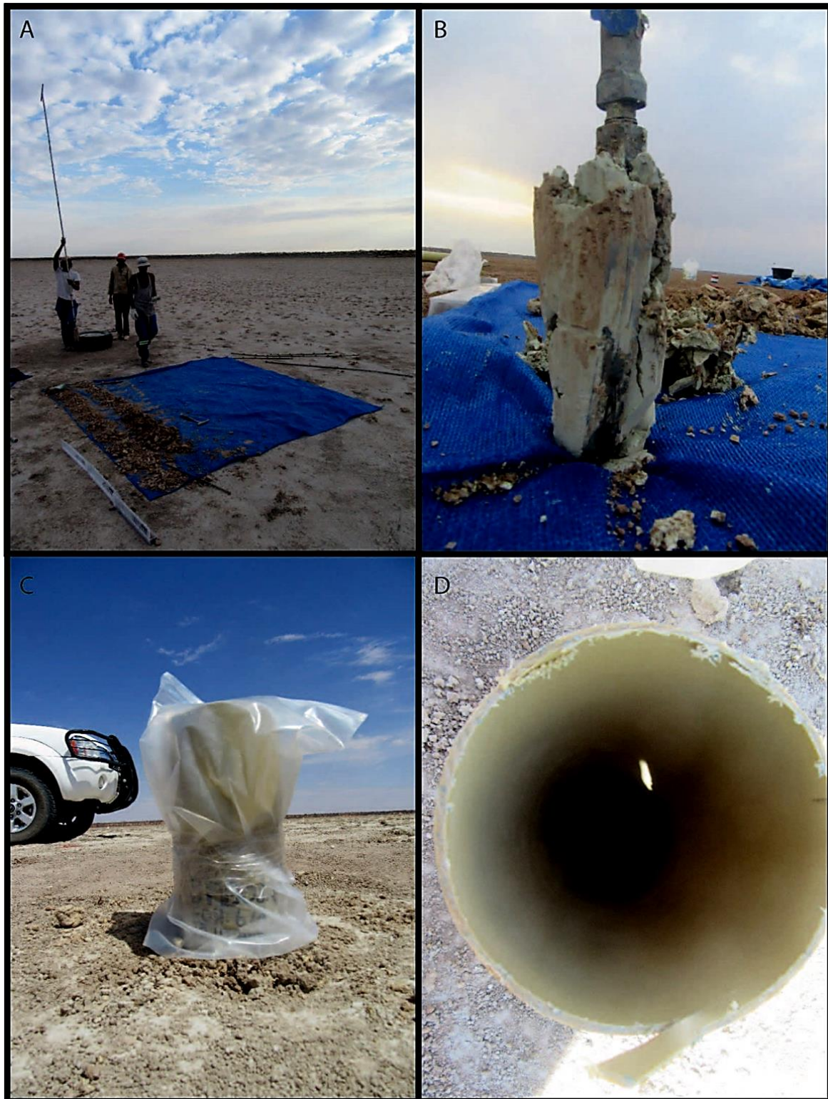
Figure 11: A – Photo mosaic of one of the drill sites, with recovered sediment sample being packed neatly on the canvas cloth as 20 cm samples. The chip-tray sample would immediately be collected and logged. B –The hand auger clay-bit together with its 20 cm interval sample. C – The collar casing which was installed at each drillhole. D – down-the-hole view of one of the drillholes, clearly indicating that the holes remain intact and stable after drilling.
