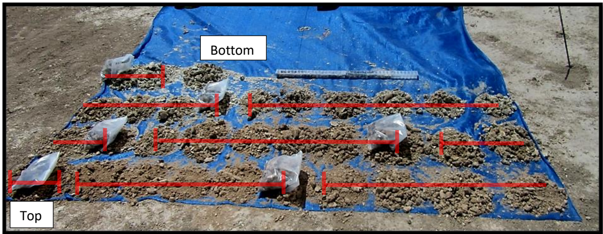
Figure 15: Example of composite sampling intervals across an auger drillhole.
