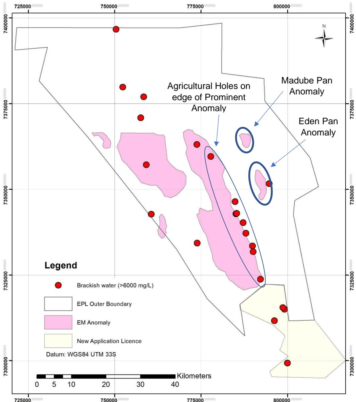
A helicopter airborne survey<sup>4</sup> commenced on 11 October 2022 consisting of 52 lines on a 1 km grid was completed over the southern and central portion of the Bitterwasser Lithium in
