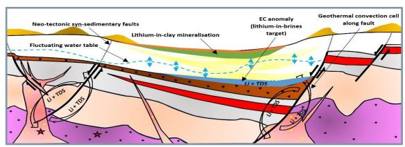
Figure: Schematic model of the Bitterwasser System to aide Arcadia's exploration for lithium-in-clay and lithium-in-brine mineralisation.
