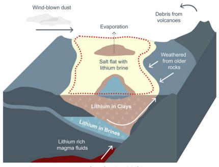
Figure: Schematic artist impression of an inferred model of the Bitterwasser Basin
