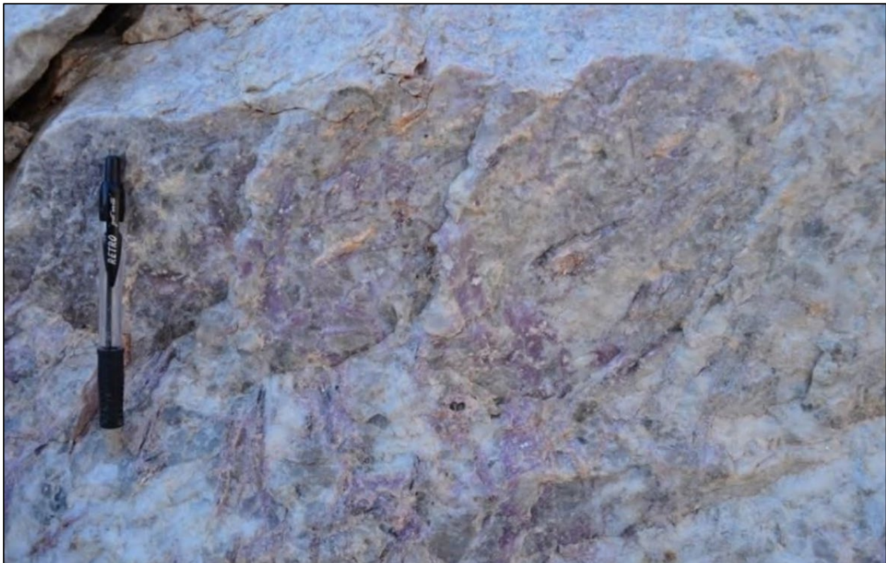
Figure 5.3 An example of mineralised D0 pegmatite clearly showing the spodumene crystals
