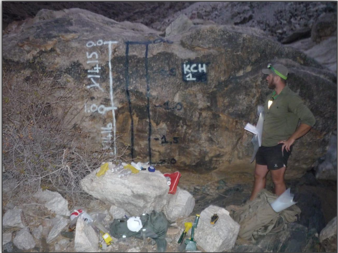
Figure 11: Marking of a channel sample in the field
