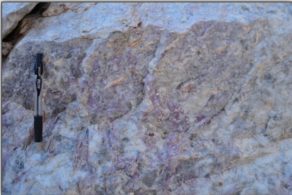
Figure 13: An example of a mineralized pegmatite face that was mapped in the field clearly showing the spodumene crystals.
