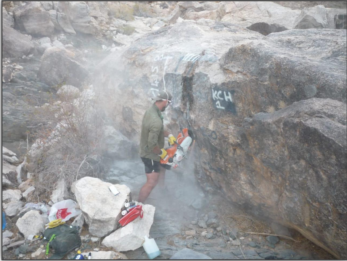
Figure 12: Cutting of a vertical channel sample
